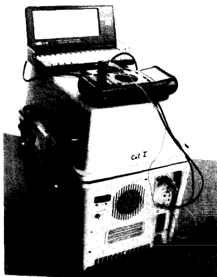
Fig. 1. Photograph of the closed direct calorimeter unit ready for operation.
